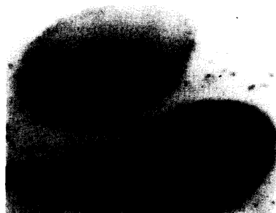
Figure 1 (a) Macrophase separated structure in a PMMA(107)/PMMA-b-PS(65) blend. Block copolymer rich domains appear dark. (b) Microphase separation within these domains is evident at higher magnification
